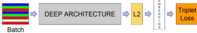
Fig. 2. Scroff et al.’s [3] FaceNet Model structure. The network consists of a batch input layer and a deep CNN followed by L2 normalization, which results in the face embedding. This is followed by the triplet loss during training.
